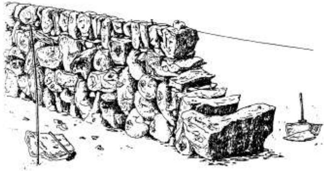
A single wall or dyke is only a single stone thick whereas the more common double wall consists of two stone walls to form the faces with small stones to fill the gap and throughstones and topstones bridging the two face walls to hold them together.
